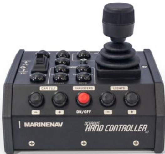
THE OCEANUS JOYSTICK / HAND-HELD CONTROLLER (v3.0)
